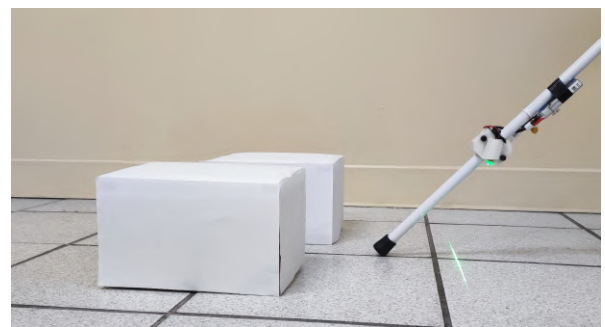
Fig. 8. Image of the first stage with two obstacles on the ground surface.
