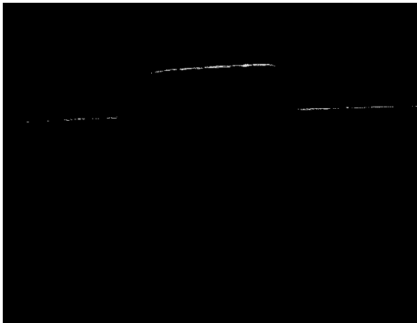
Fig. 10. The image that shows what the camera sees when passing through an obstacle is the line seen above, and it has different filters to focus on the reflection that the laser beam hits the ground and the obstacle.
