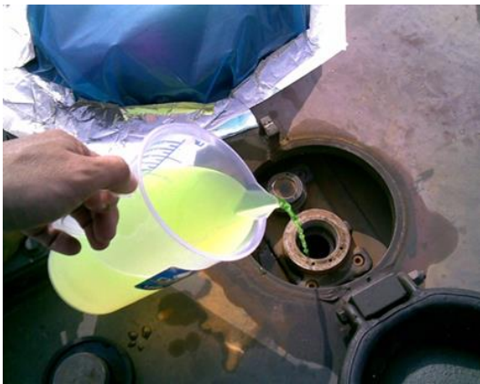
Figure 5-5: Preservation of cooling system using VCI coolant additives
