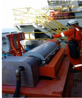
Figure 5-13: Preservation of hydraulic system using VCI hydraulic oil additive
