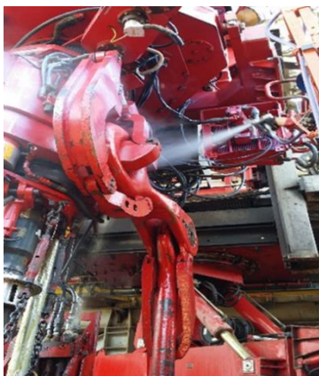
Figure 5-14: Apply VCI acrylic coating to the exterior equipment
