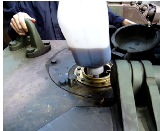
Figure 5-7: Preservation of fuel systems using VCI fuel additives
