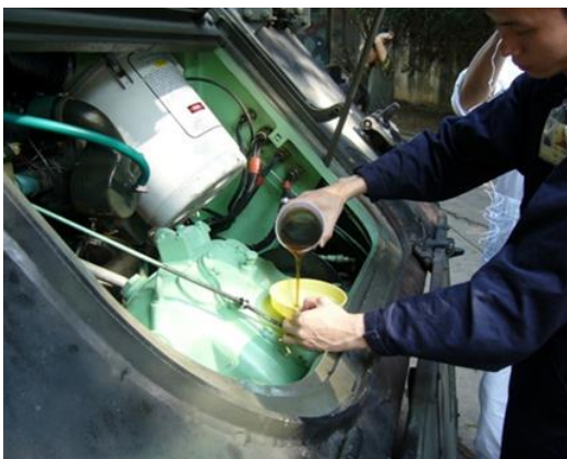
Figure 5-6: Preservation of engine system using VCI engine oil additive
