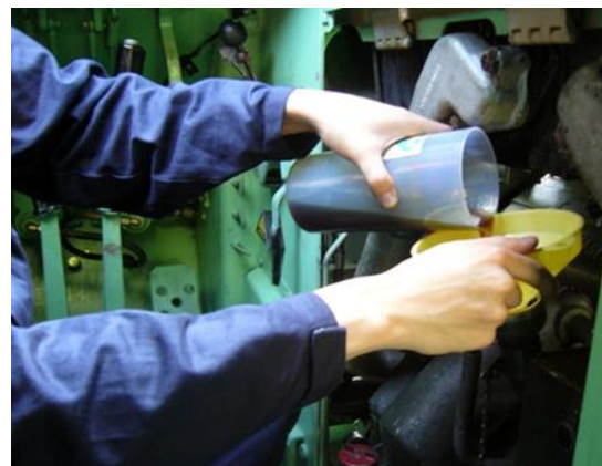
Figure 5-6: Preservation of engine system using VCI engine oil additive
