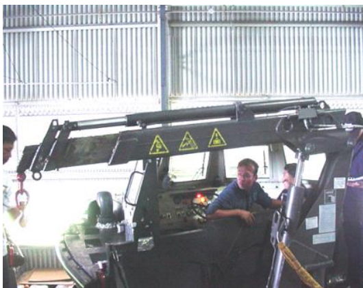
Figure 5-9: Preservation of hydraulic systems using VCI hydraulic oil additive
