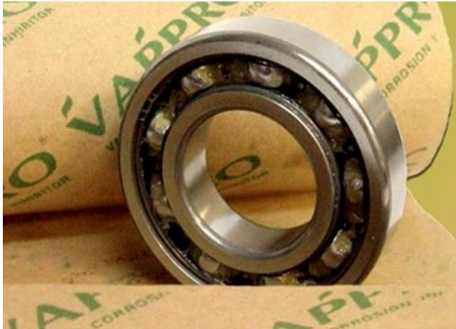
Figure 4-18: Machinery part packed with VCI paper
