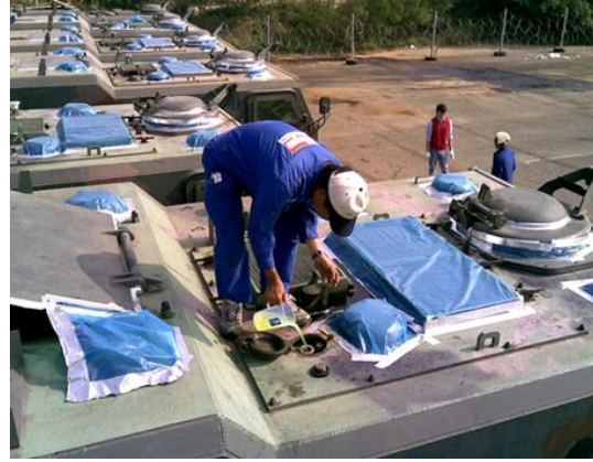
Figure 5.4: Preservation of armoured vehicles with VCI plastic
