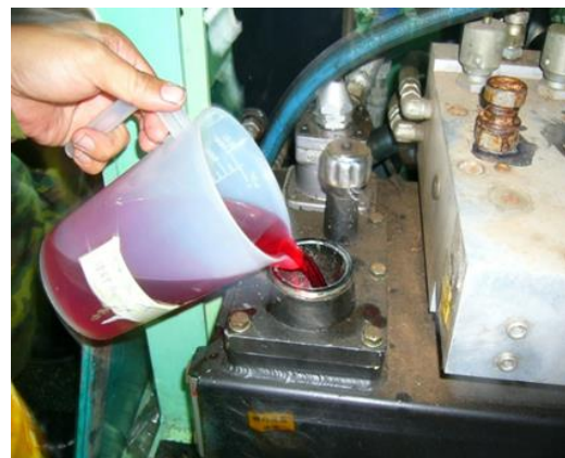
Figure 5-9: Preservation of hydraulic systems using VCI hydraulic oil additive
