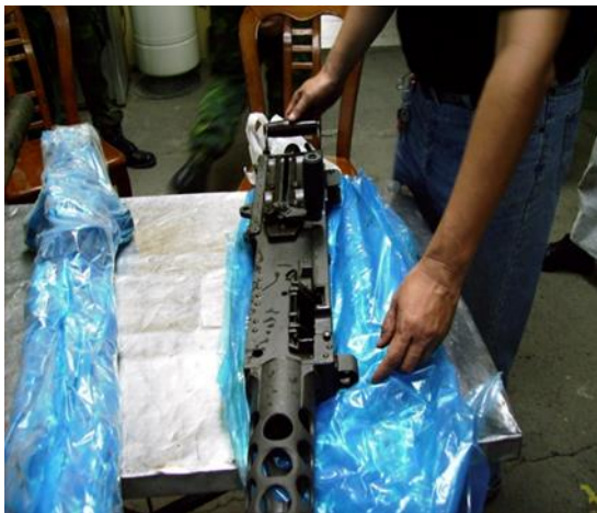
Figure 4-15: VCI film used in military weapons
