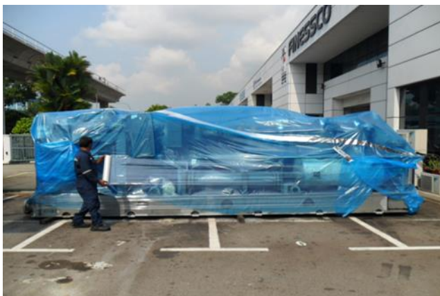
Figure 3-4: VCI plastic used to prevent corrosion of spare parts during shipping and storage.
