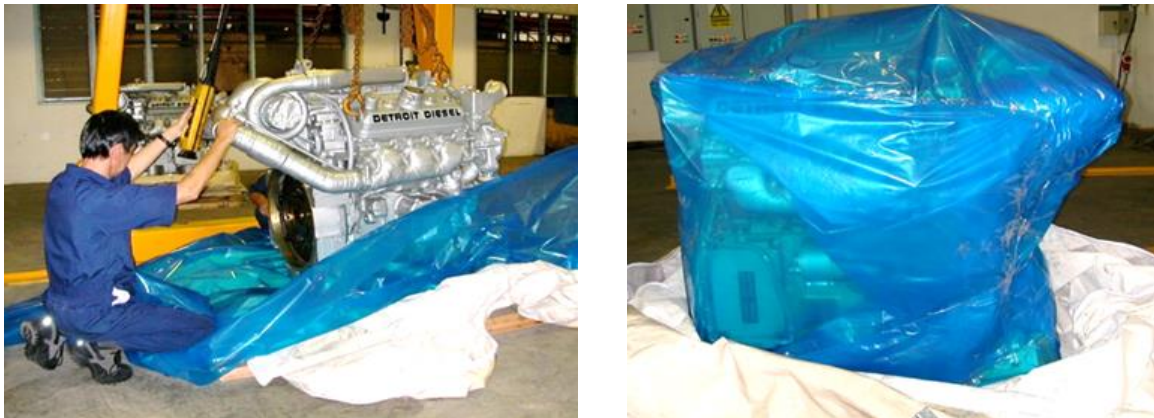
Figure 5-21: Protection of engine with VCI film
