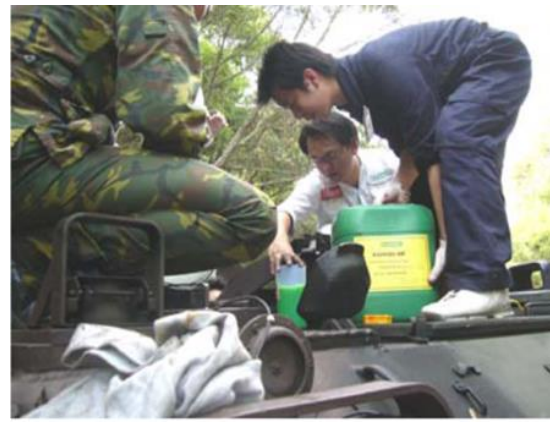
Figure 5-5: Preservation of cooling system using VCI coolant additives
