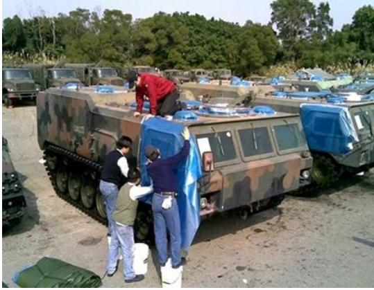
Figure 5.4: Preservation of armoured vehicles with VCI plastic
