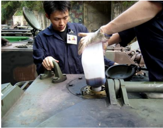
Figure 5-7: Preservation of fuel systems using VCI fuel additives
