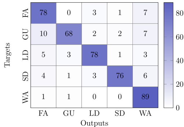
Figure 6.20: Confusion matrix obtained for the embedded model with uint8 quantization, x8 data augmentation, and variance-based subcarrier selection.
