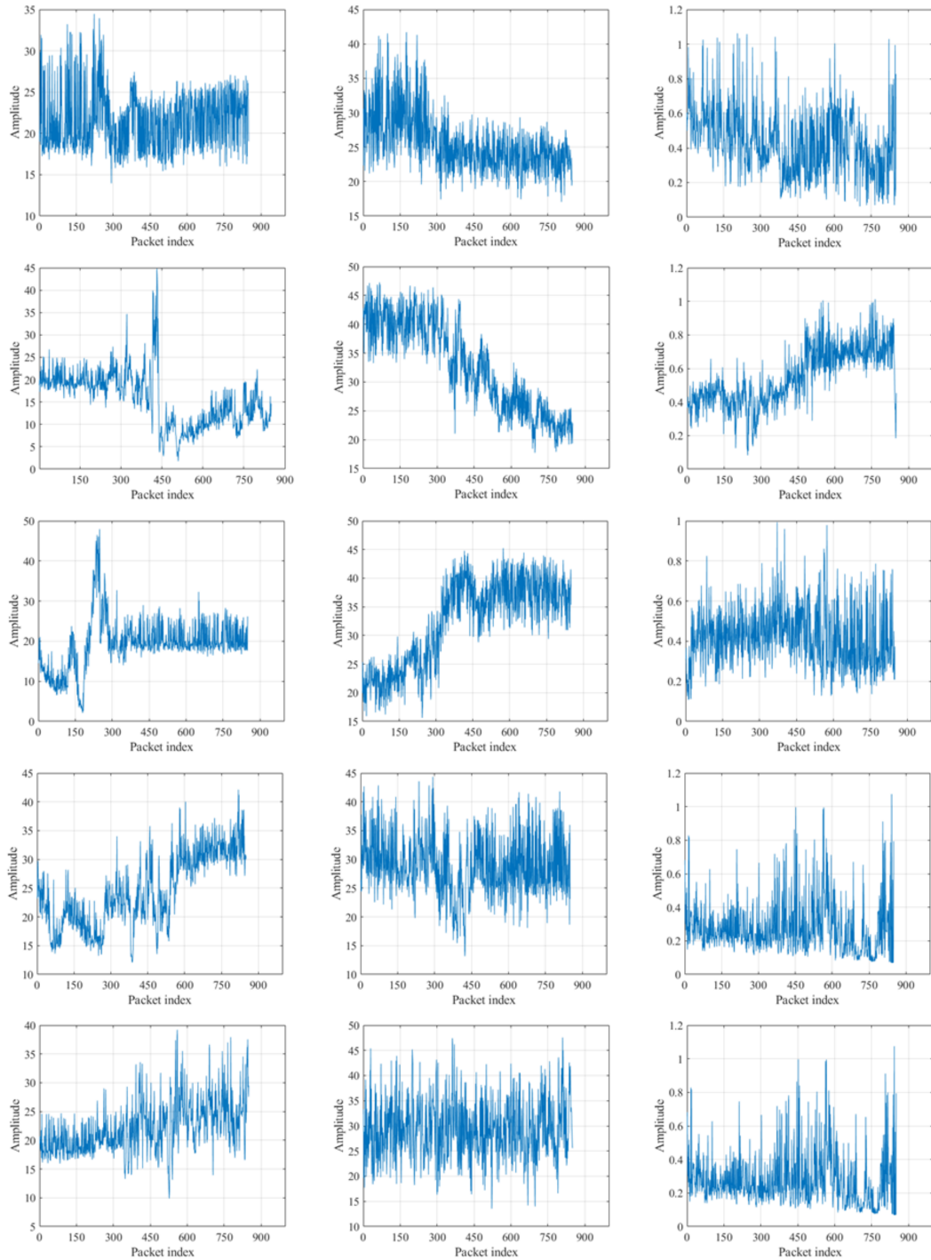
Figure 6.5: From left to right, original subcarrier amplitude, synthetic amplitude generated with the EMD-based algorithm, and synthetic amplitude generated with DCGAN. From top to bottom, fall, get up, lie down, sit down, and walk.
