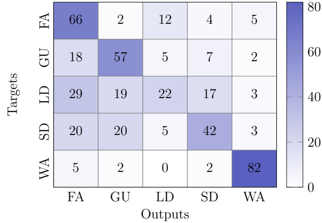
Figure 6.15: Confusion matrix for activity classification with no data augmentation
