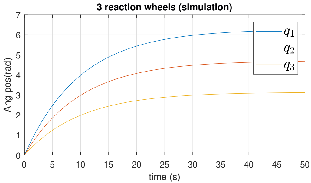
Figure 5.23: 3-dof simulation angular position. The body is initially at rest. and the simulation runs from t = 0 to t = 50 s. The desired final positions were q_1 = 2\pi q_2 = 3\pi/4 and q_3 = \pi rad. The block diagram of this simulation is presented in Figure E.3 .
