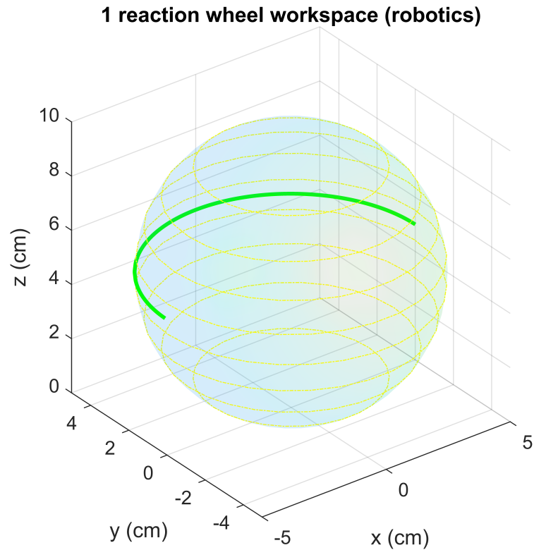
Figure 5.7: 1-dof theoretical model workspace (3D view with robotics). The body is initially at rest. The green line is the trajectory of the final framework from t = 0 to t = 50 s. The desired final position was \pi rad. The block diagram of this simulation is presented in Figure E.4
