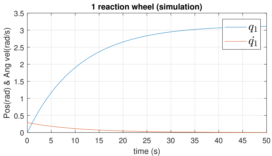
Figure 5.6: 1-dof angular velocity and angular position. The body is initially at rest and the simulation runs from t = 0 to t = 50 s. The desired final position was \pi rad. The block diagram of this simulation is presented in Figure E.1 .
