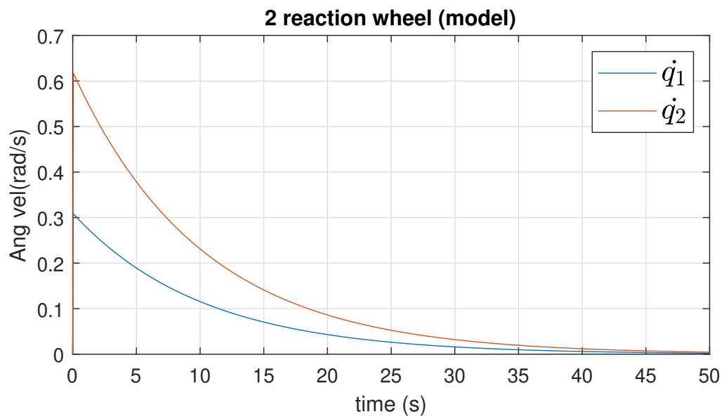
Figure 5.12: 2-dof theoretical model angular velocity. The body is initially at rest, and the simulation runs from t = 0 to t = 50 s.
