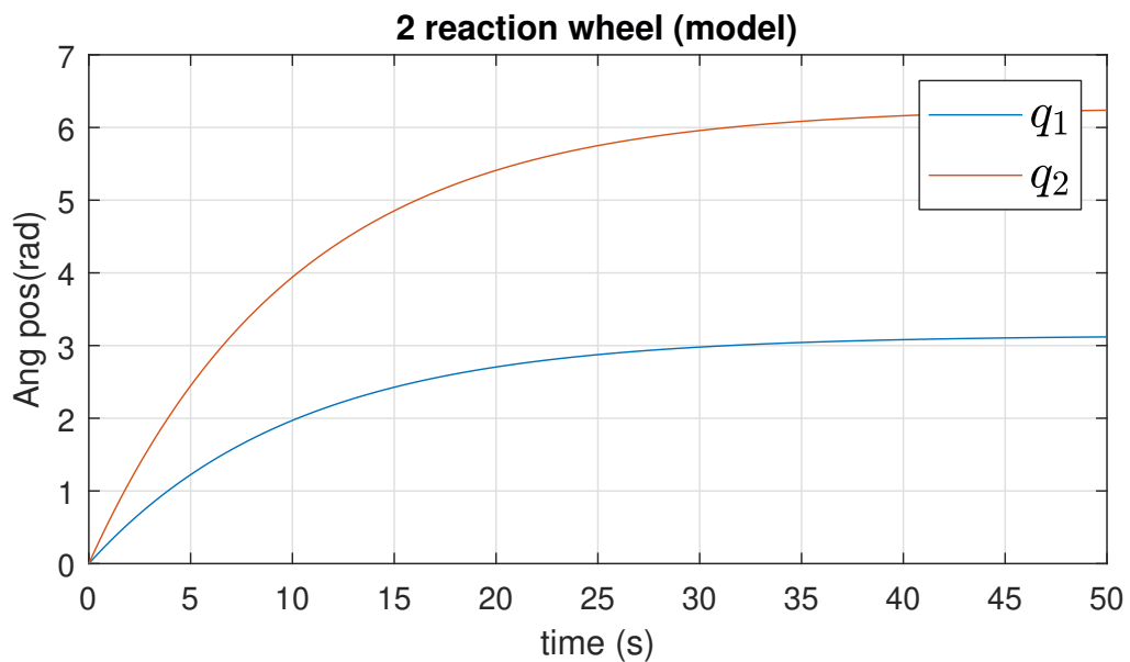
Figure 5.11: 2-dof theoretical model angular position. The body is initially at rest, and the simulation runs from t = 0 to t = 50 s. The desired final positions were q_1 = \pi and q_2 = 2\pi rad.
