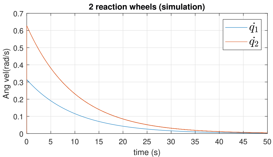
Figure 5.15: 2-dof simulation angular velocity. The body is initially at rest, and the simulation runs from t = 0 to t = 50 s. The desired final velocities were \dot{q}_1 = \dot{q}_2 = 0 rad. The block diagram of this simulation is presented in Figure E.2 .
