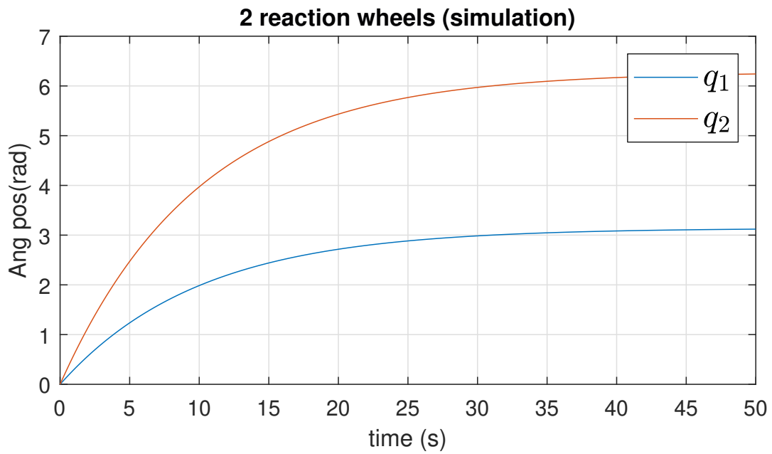
Figure 5.14: 2-dof simulation angular position. The body is initially at rest, and the simulation runs from t = 0 to t = 50 s. The desired final positions were q_1 = \pi and q_2 = 2\pi rad. The block diagram of this simulation is presented in Figure E.2 .
