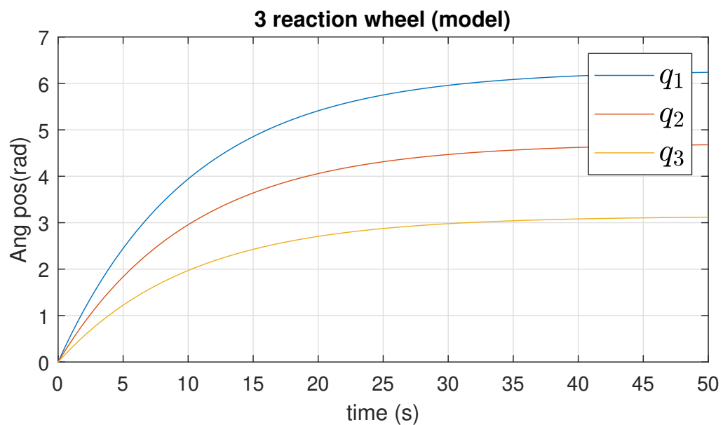
Figure 5.20: 3-dof theoretical model angular position. The body is initially at rest. and the simulation runs from t = 0 to t = 50 s. The desired final positions were q_1 = 2\pi q_2 = 3\pi/4 and q_3 = \pi rad.
