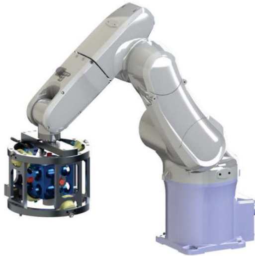
Figure 2.11: CubeSat testbed airBall prototype with a robotic arm manipulator. Taken from Gavrilovich (2016).
