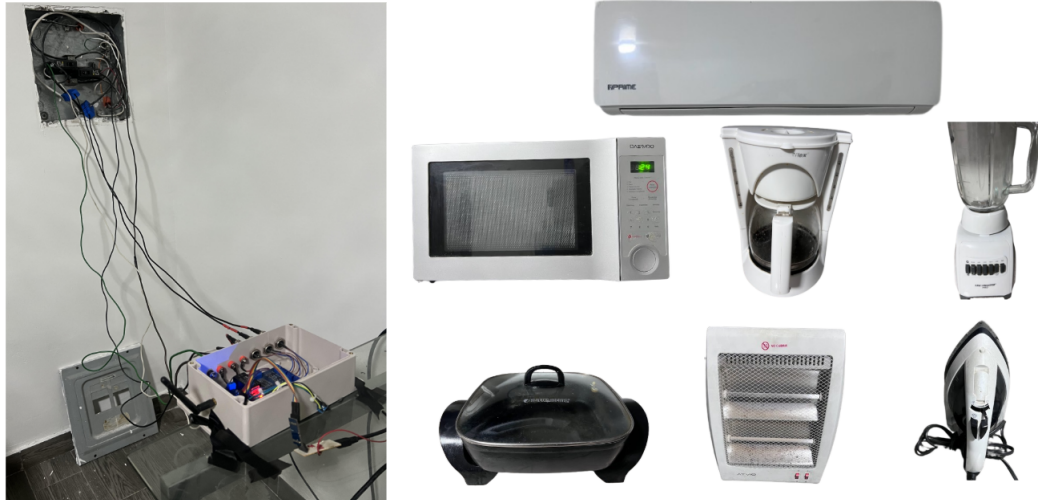
Figure 5.1: Testing environment: Smart meter installation and appliances used.
