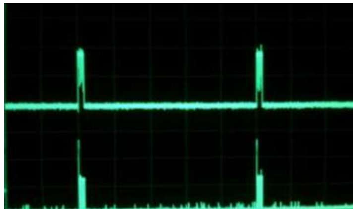
Figura 13. SI = 250 ms, t/Div=100 ms, V/Div: V_{out}=500\text{mV} , SI=1V, CLK=2V.
