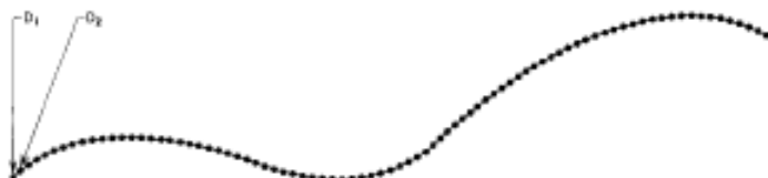
Figure 2 Curve defined by linear segments joining data points
