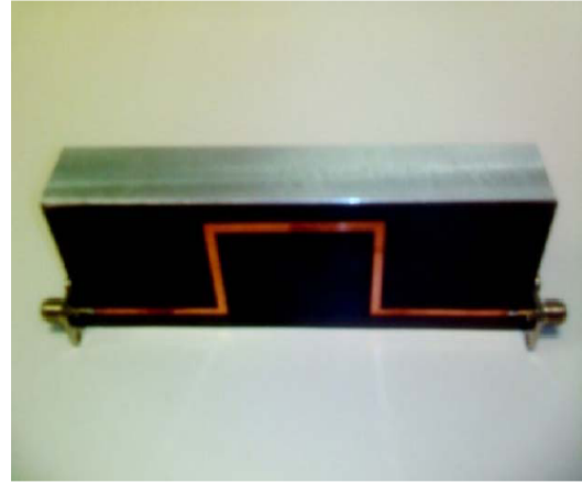
Fig.1 Photograph of a single-loop microstrip delay line constructed on a substrate of 0.07874 cm of thickness with a relative permittivity of 2.2 and double terminated in SMA female connectors.
