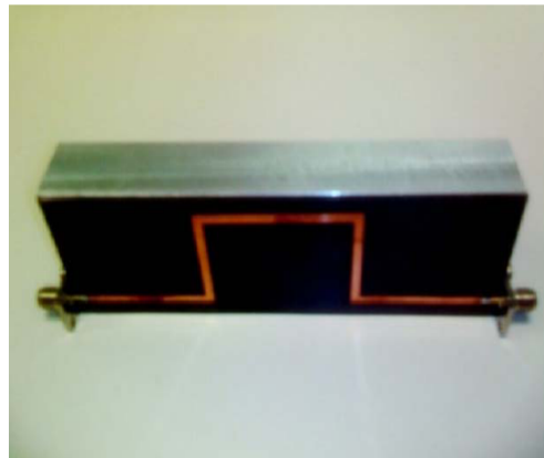
Fig.1 Photograph of a single-loop microstrip delay line constructed on a substrate of 0.07874 cm of thickness with a relative permittivity of 2.2 and double terminated in SMA female connectors.
