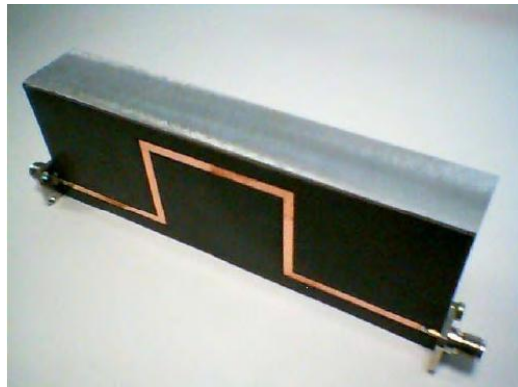
Fig. 3. Photograph of a single-loop microstrip delay line constructed on a substrate of 0.07874 \text{ cm} of thickness with a relative permittivity of 2.2 and double terminated in SMA female connectors.
