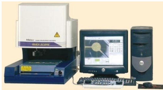
Figura 1.9 Quick Scope 200Z de Mitutoyo
