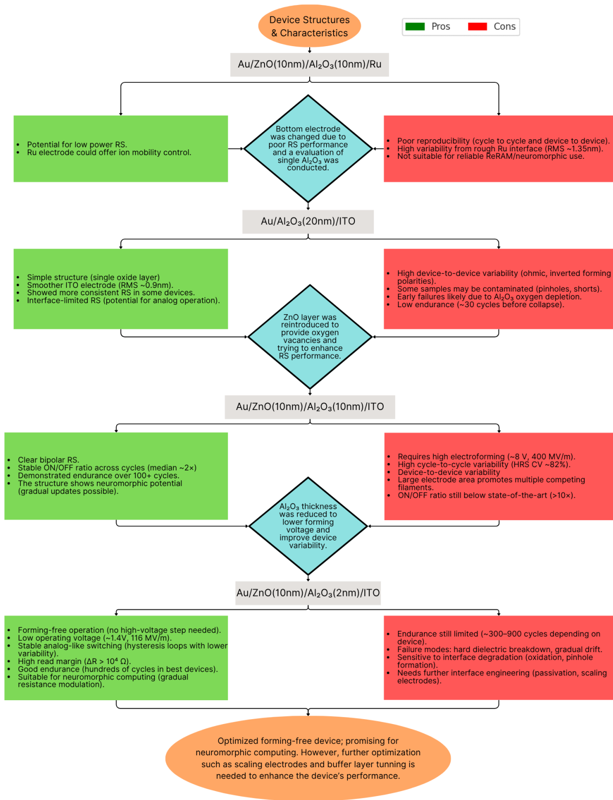
Fig. 10 | Flow chart of the device's structures and characteristics.
