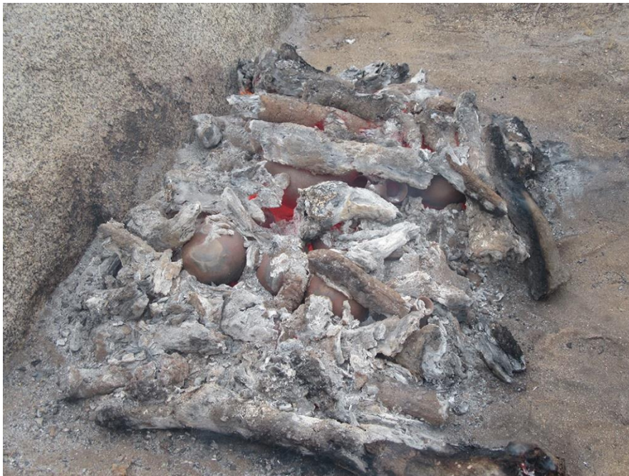
Figure 36. Forty-five minutes after the fire had begun, the fuel was nearly reduced to ash and embers. May 6, 2017.
