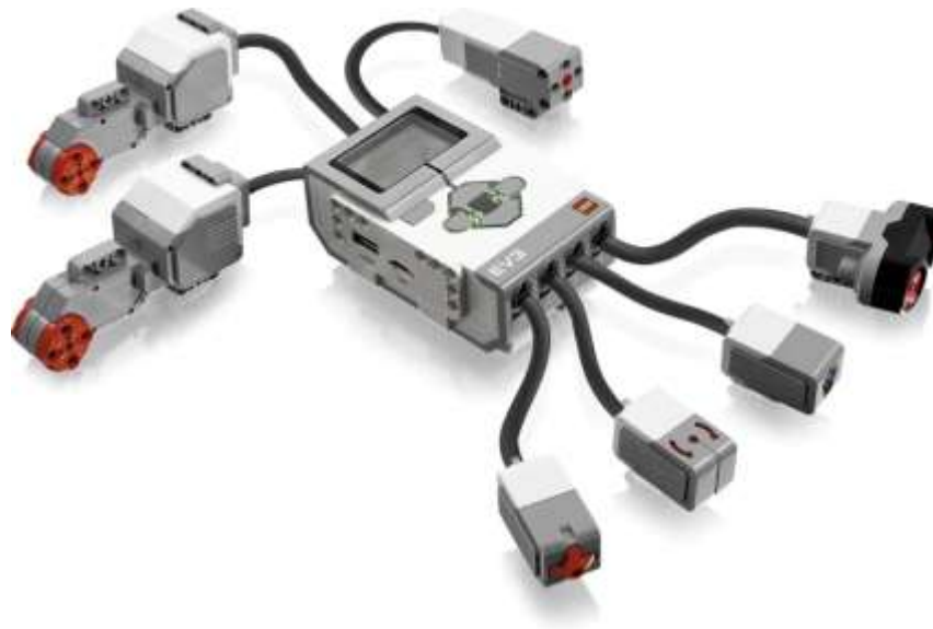
Figura 2.32: Kit robotica LEGO Mindstorms EV3
