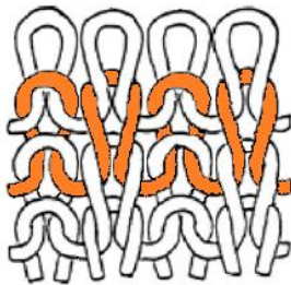
Figure 1. Rib knitted structure. Source: [1]. The authors.
