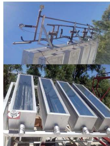
Fig. 6. CPC solar collector test bench constructed and installed in Mexicali, Mexico
