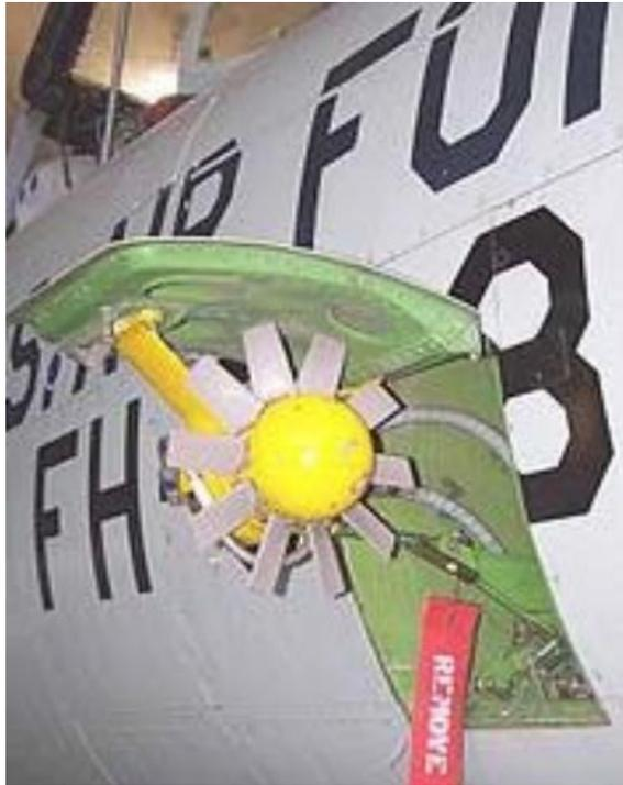
**Figure 1.1.** RAT for military application on a USAF F-105 (Bolognesi et al., 2009).
