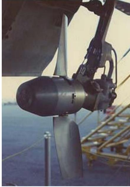
**Figure 1.2.** RAT in commercial application on BOEING 757 (Bolognesi et al., 2009)
