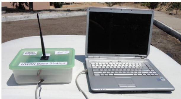
Fig. 2.2.3.9. Base station and crossover connection to the portable DBS server.
