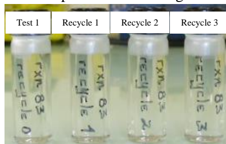
Figure 6.13 Liquid reaction mixtures obtained by filtration after the recycling tests. Reaction time for all cases: 3 h.
