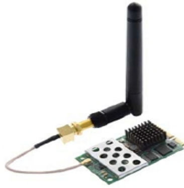
Figura 4.1: Módulo Rabbit MiniCore RCM5600W
