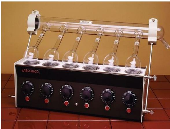
Figura 5. Digestor LABCONCO
