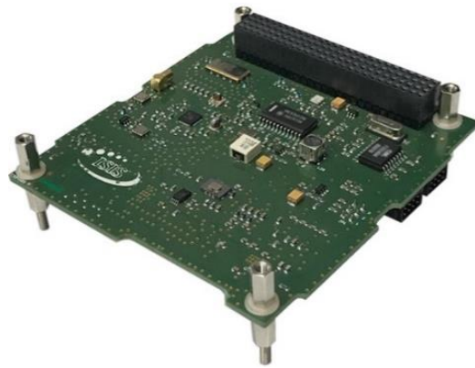
Figura 19 ISIS UHF uplink/VHF downlink Full Duplex Transceiver [57]
