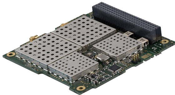
Figura 20 ISIS VHF uplink/UHF downlink Full Duplex Transceiver [58]
