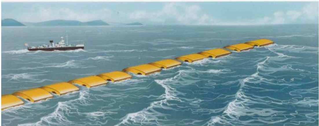
Figure 8. Salter's nodding-duck shaped bodies, performing pitch oscillation, with different phases [35].
