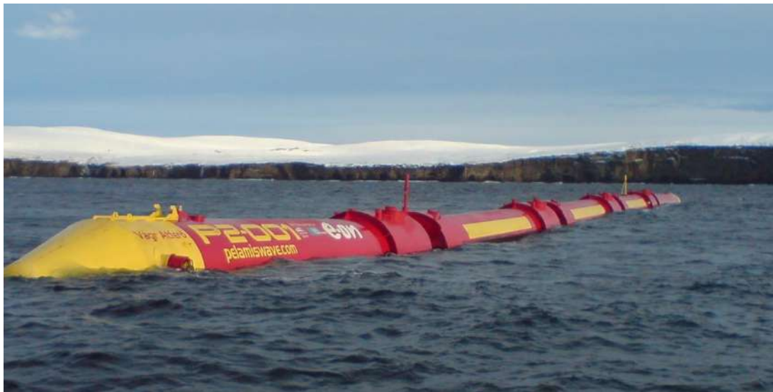
Figure 9. Pelamis Wave Power, an example of an attenuator device [38].
