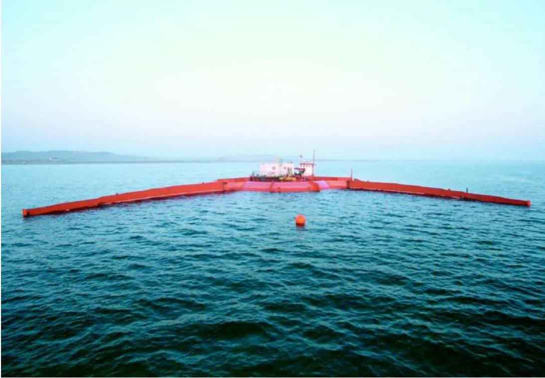
Figure 6. The WaveDragon overtopping device [33].
