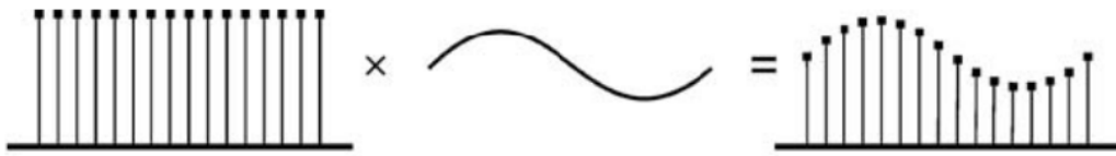
Figure 2.14: Illustration of the sampling process as a product of subsequent impulses sampling the continuous phenomenon and producing a discrete signal representing it, as presented by [8].
