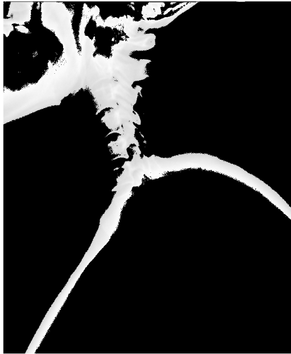
Figure 4.7: Mask generated from Figure 4.4 where values between 63 941 (minimo + 1500) and 64241 (minimo + 1800) are kept and the rest is assigned the minimum value, in this case 62441.
