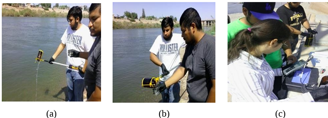
Figure 3.3 Samples collection. (a) rinsing the bottles before taking the sample; (b) and (c) measurement of physicochemical parameters.
