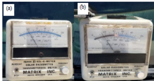
Figure 1. Radiometer a) without solar film, b) with solar film.
