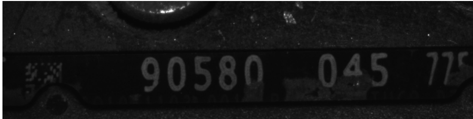
Figure 3.17: OCR Digits Damage with superficial dirt in lower locations.
