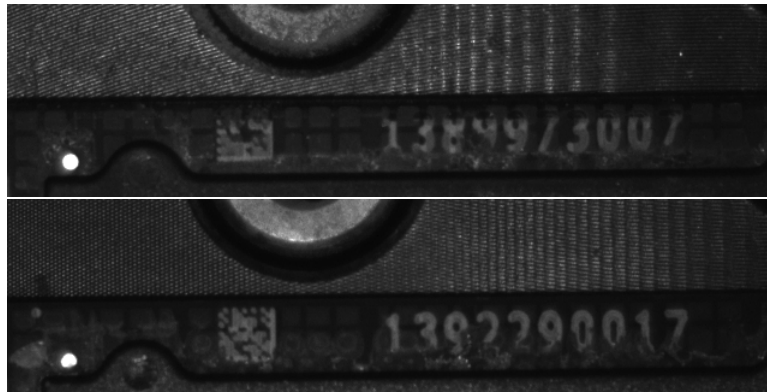
Figure 4.16: PCBs with evident residual dirt over characters.
