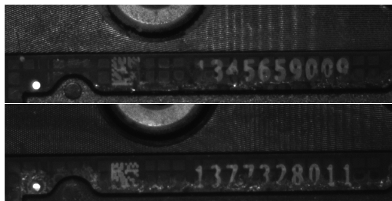
Figure 4.23: PCBs with evident residual dirt over characters.
