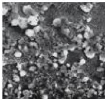
Figure 2. SEM micrograph of the nanocomposite sensitive layer (20% \text{SiO}_2 nanoparticles in olive oil) deposited on the conductometric electrode surface. Scale: 1000 nm \text{cm}^{-1} .
