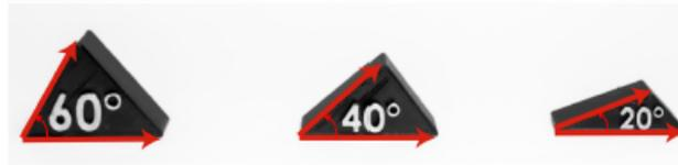
Fig. 6. Test 1 Bases, with inclinations 20°, 40° and 60° for the estimation of initial orientation conditions.
