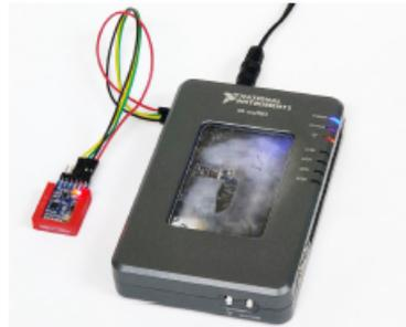
Fig. 5. Equipment and instrumentation National Instruments MyRIO acquisition system and MPU-9255S.
