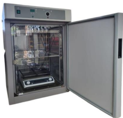
Figura 13. Incubadora (VWR International Model 1545).
