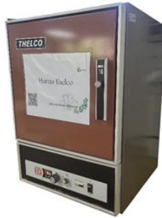
Figura 11. Horno de secado (Thelco Precision Scientific Incubator Oven 31480 Model 16).
