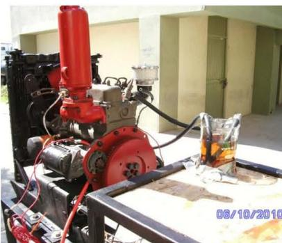
Figura 2. Motor diesel 3 pistones
