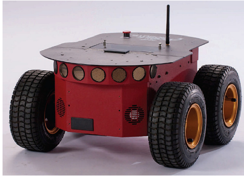
Fig. 6. Pioneer 3-AT mobile robotic platform.
