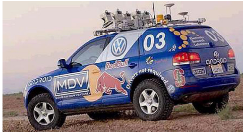
Fig. 1. Stanley—the Stanford Autonomous Vehicle that won the DARPA Grand Challenge.
