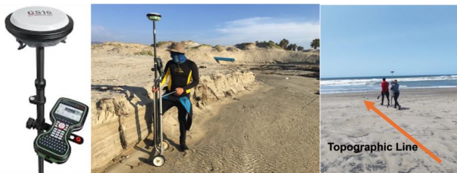
Figure. 2.2.1.1. Topographic data collection using RTK-GPS on foot using a two-wheeled pole.
