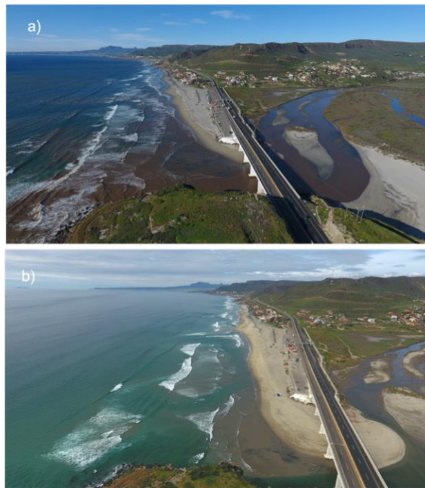
Figure 2.6.6. Aerial views of La Misión beach taken from UAV imagery. (a) Inlet opened on 2 nd of March 2017. (b) Inlet closing in 21 st March 2017. Note the input of sediments in (a) towards the beach, and the presence of wide rip currents in (b).
