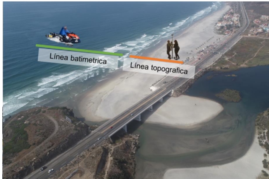
Figure. 2.2.3.3 Schematic diagram of the instruments used for the subaerial and subtidal morphological data collection at La Misión Beach.
