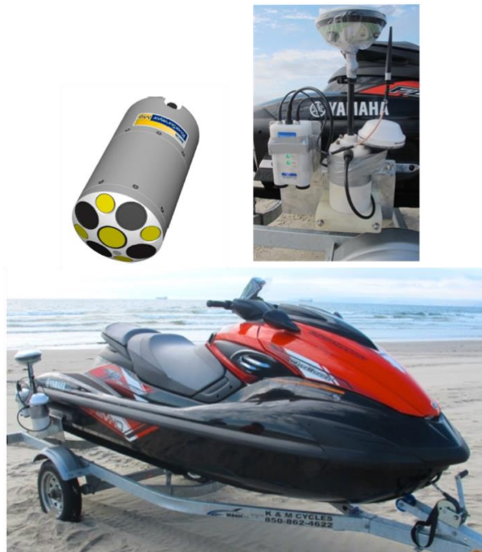
Figure. 2.2.2.2 Equipment used for the collection of bathymetric data. Example of the Sontek M9 echo-sounder integrated on an ADCP (top left panel) and the equipment mounted onto the jetski (top right and bottom panels).
