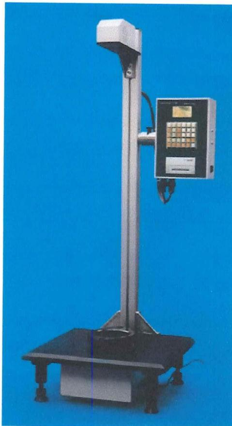
Figura 29. BMC-B1 falling dart impact tester
