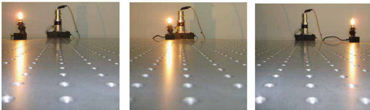
Fig. 11. Measurements angle and distance representation (Angle of Scanning every 5° and Distance of Scanning every 1 cm).
