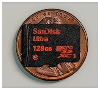
Figura 2.47: tarjeta microSD (Lady-ada, 2017)
