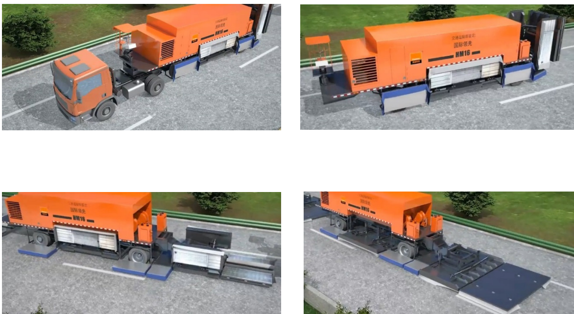
Figura 53. Máquina HM16 paneles desplegables (Freotech, 2014)
