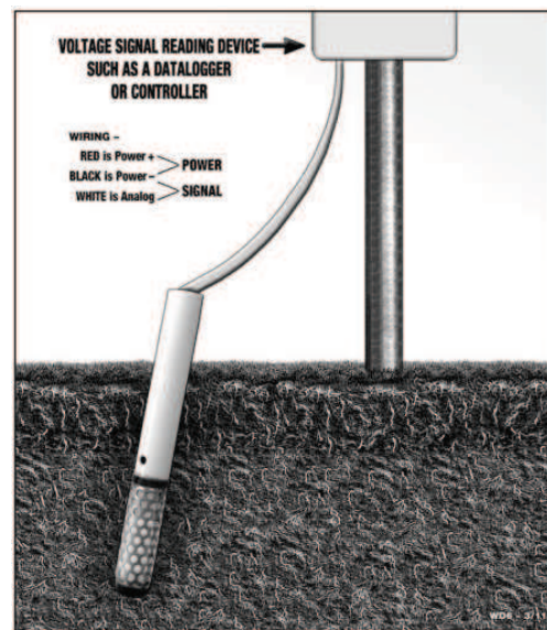
Figura 4.1: Alambrado del sensor Watermark 200ss-v.
