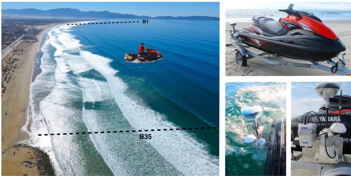
Figure 2.5 Aerial image of the beach (left panel). The dashed lines represent the first and last bathymetric lines out of 35 surveyed. The equipment used to carry out the measurements is presented in the right panels: jetski equipped with an ADCP and the RTK-GPS.
